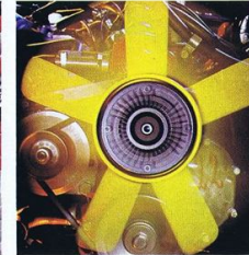
New fan with slip-type coupling which maximizes fan speed to 3,500 r.p.m.
